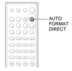
Press AUTO FORMAT DIRECT on the remote repeatedly until "A.F.D. AUTO" appears in the front panel display.
